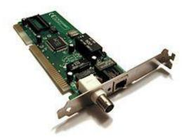
4. **Ethernet Card:** Ethernet card is used to connect computers to computers. A cable is used to connect the Ethernet cards in each computer to make a network.
