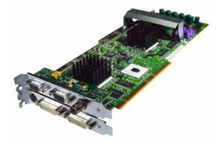
6. **Video Capture Card:** This card is used to convert analog signals (signals from video camera or VCR) to a compressed digital signal. This compressed digital signal can be stored in your computer as a video file.
