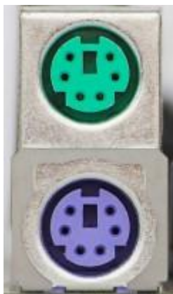
PS/2 Ports, green for mouse and purple for keyboard
