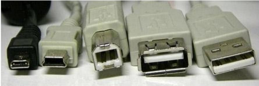
*From left to right: micro USB, mini USB, type B standard USB, and type A standard USB (both female and male).*
