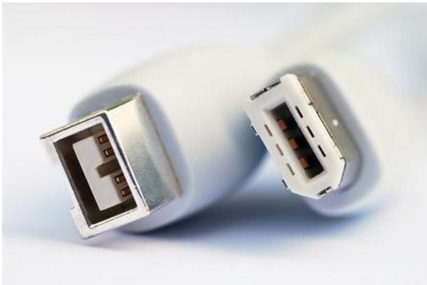
The purpose of FireWire is similar to that of USB: high speed data transfer for computer peripherals. High bandwidth devices, like printers and scanners, will benefit from FireWire. For whatever reason, FireWire is not as widespread as USB. FireWire cables come in two forms: 1394a (which has a transfer speed of 400 Mbps) and 1394b (which has a transfer speed of 800 Mbps).
