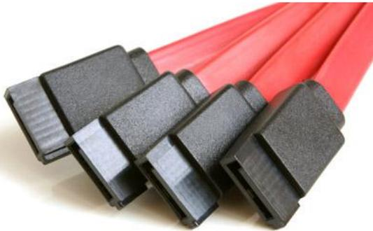
Newer hard drives will likely use SATA ports over IDE ports. In fact, SATA was designed to succeed IDE, and it has. Compared to IDE, SATA provides higher data transfer speeds. Your motherboard needs to be compatible with SATA, and nowadays most of them are.
