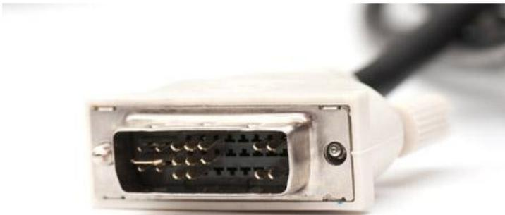
The DVI connection became the successor to VGA as technology moved away from analog towards digital. Digital displays, like LCD, proved to be higher quality, which soon became the market standard for home pictures. DVI connectors come in 3 varieties.
