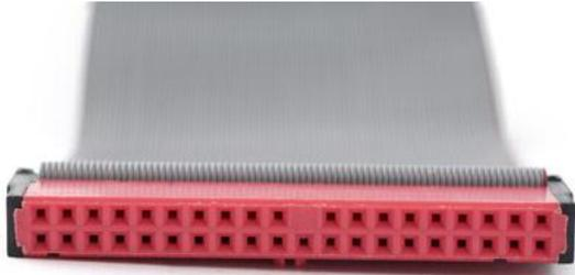
IDE cables were used to connect storage devices to a motherboard. If you've ever opened up an old hard drive then you likely know what an IDE connector looks like. It's the wide cable that looks like a ribbon with more than 2 plugs.
