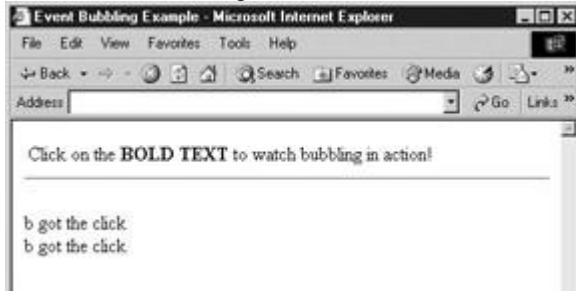
Figure 11-2: If an event is cancelable, setting event.cancelBubble prevents the event from propagating.
