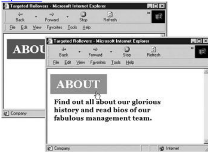
Figure 15-2: Updating a separate region of the document in response to a rollover
